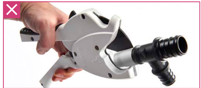
Fig. 5.8: DO NOT cut RAUPEX pipe from fitting
